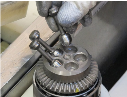
14. Assemble the pistons. Lubricate the ball sockets before assembly.
