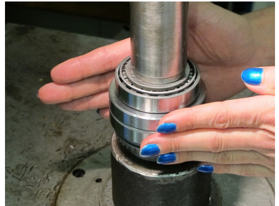
5. Press down the small tapered roller bearing in small steps until correct preload is achieved. Not too tight and no backlash.
