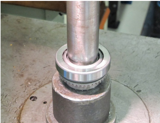
2. Press down the big tapered roller bearing together with the ring gear.
