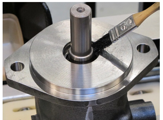
18. Lubricate the sealing surface on the shaft before assembling the shaft seal.
