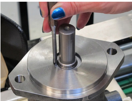
21. Carefully tap down shaft seal and support ring.
