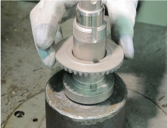
1. Place the ring gear on the shaft with the guide pin located against the guide hole.
