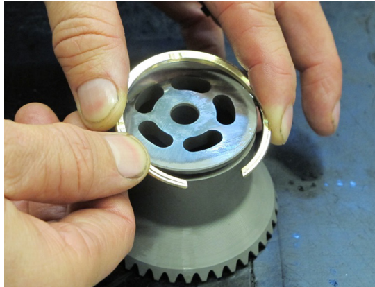
1. Assemble the barrel retaining ring. Note, grooves upwards as on picture.
