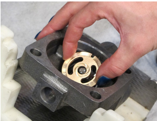
9. Assemble the valve plate. Make sure the slot is in correct position and the valve plate is located as shown in picture.
