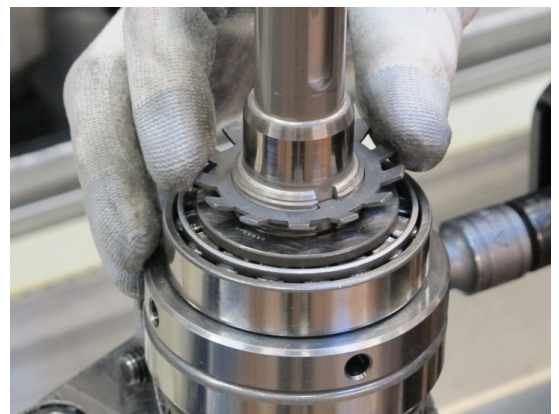
6. Place the lock washer(s) on to the shaft.
