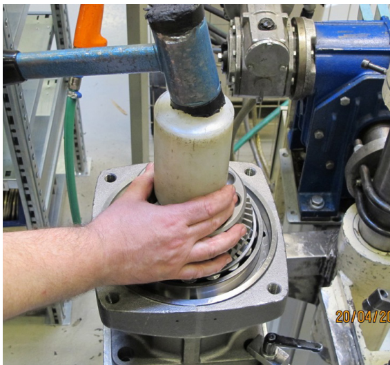
5. Tap down the bearing package into the bearing housing (item 211) by using a plastic collar and a plastic hammer.
