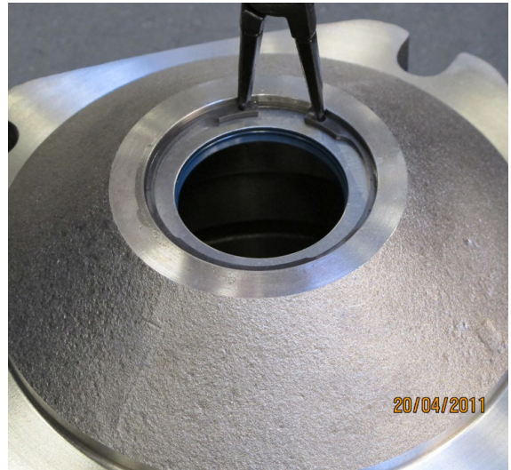
11. Assemble the retaining ring (item 237). Lubricate the shaft seal before assembling the housing.
