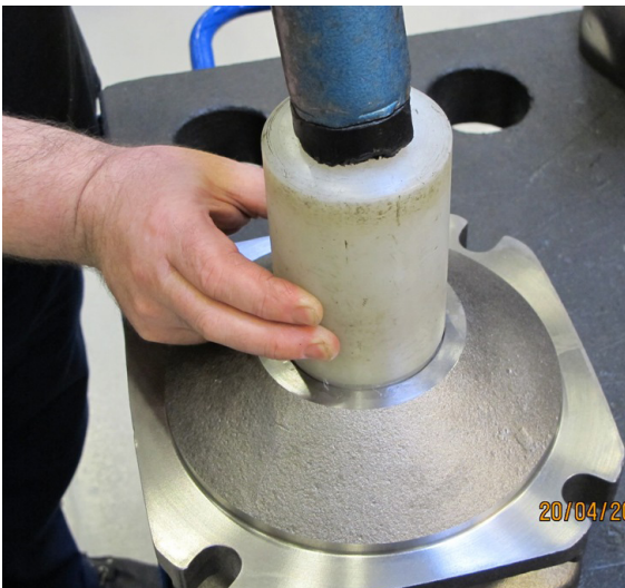
10. Assemble the shaft seal (item 233) and the support ring (item 236). Locate the chamfer on the support ring downwards. Tap it down with a plastic collar.
