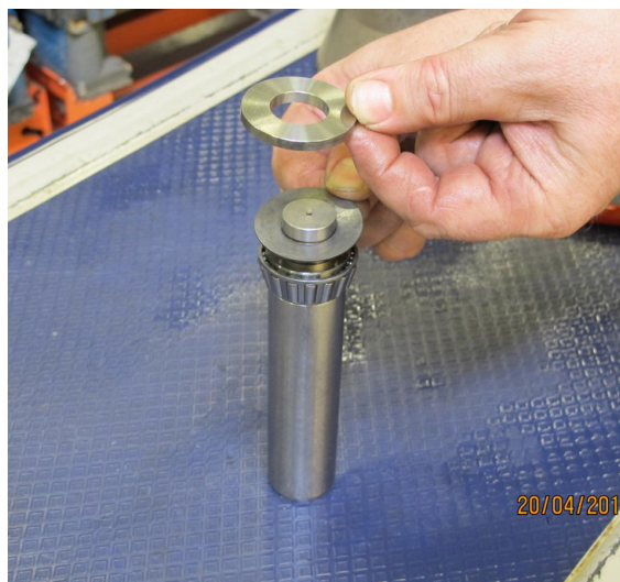
7. Assemble the tap roll bearing (item 425), the disc spring (item 433), the spacer washer (item 426) and the retaining ring (item 427).
