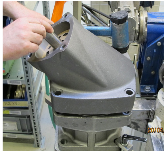
11. Assemble the barrel housing. Make sure the cylinder barrel is in correct position by holding the barrel spindle (item 423). Tap the housing down with a plastic hammer.
