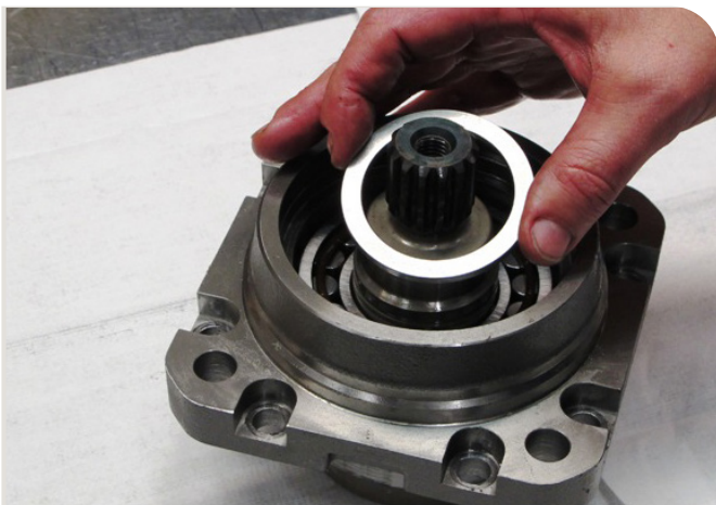
3. Assemble the bearing ring with the text downwards.
