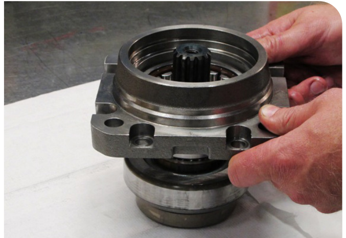
2. Press down the roller bearing with the text upwards into the flange and assemble it on the shaft package.
