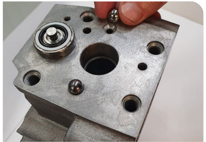
35. Assemble the check valve balls.
