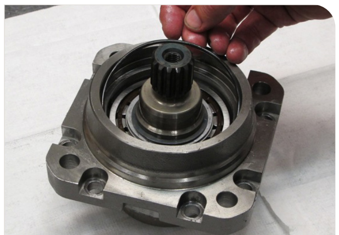
6. Assemble the O-ring.
