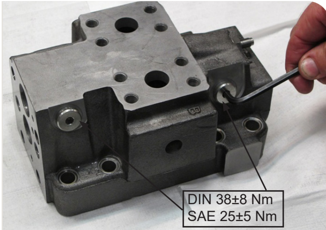
19. Assemble the hexagon plugs.
