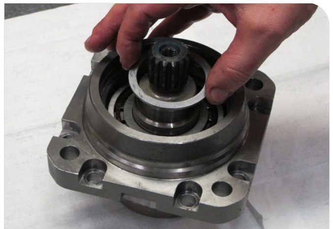
4. Assemble the shim.
