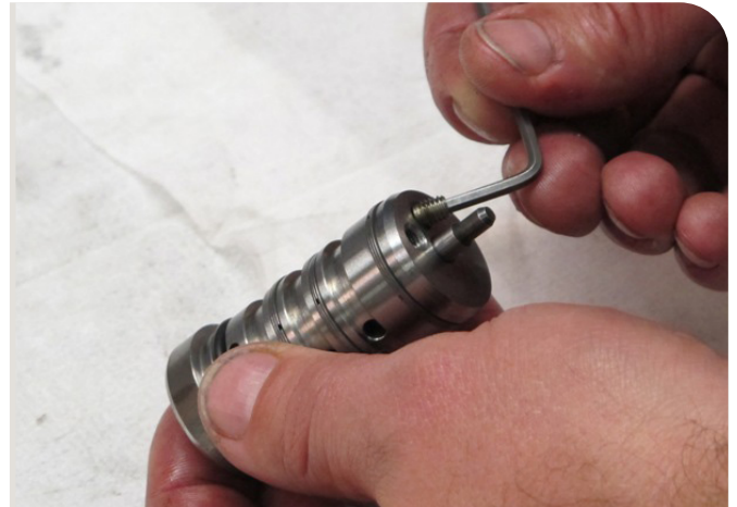
32. Assemble the nozzles and torque them to 1,2 \pm 0,2 Nm.
