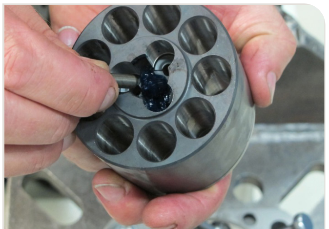
47. Assemble the support pin. Use a lot of grease to keep it in place.
