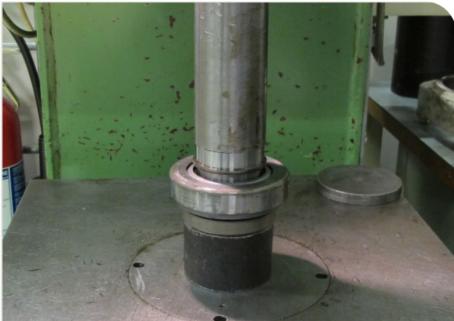
1. Press down the big tapered roller bearing and the inner ring for the roller bearing in two steps.
