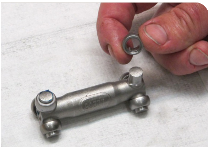
11. Assemble the joint rollers on the joint shaft. Make sure the step on the joint rollers is fitted inwards.
