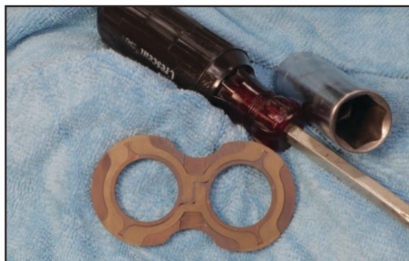
Figure 16 - Motor Pressure Plate - Seal in Place
