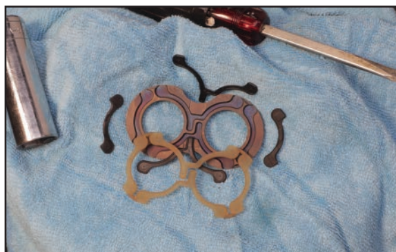
Figure 15 - Motor Pressure Plate - Back Side
