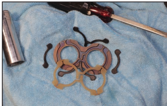
Figure 13 - Pump Pressure Plate - Back Side
