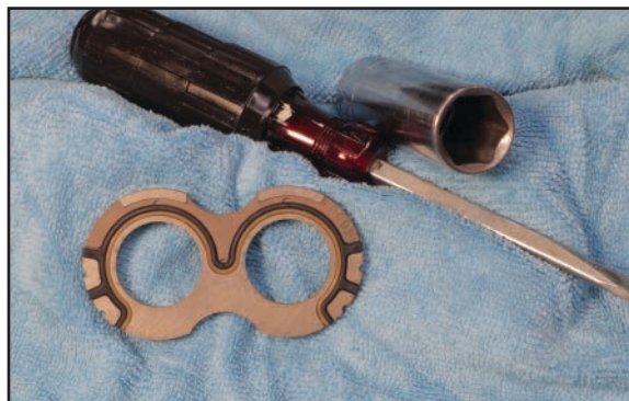
Figure 14 - Pump Pressure Plate - Seal in Place
