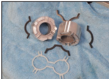
Figure 17 Pump Thrust Block - Back Side
