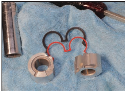
Figure 14 Pump Thrust Block - Back Side
