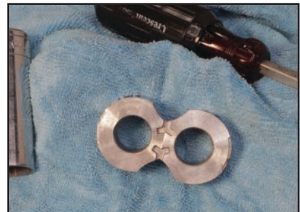
Figure 19 Pump Thrust Block - Front Side
