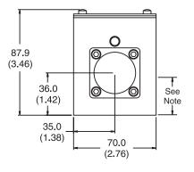
Note: 30.0mm (1.18") from bottom of bolt hole counterbore to bottom of valve.
