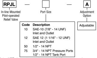
Note: NPT pipe ports are not recommended for pressures above 138 Bar (2000 PSI)
