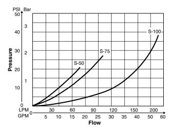
**Note:** Model S selectors will tolerate flow rates well in excess of those shown here. Consideration should be given to the restrictiveness of the port adaptors.
