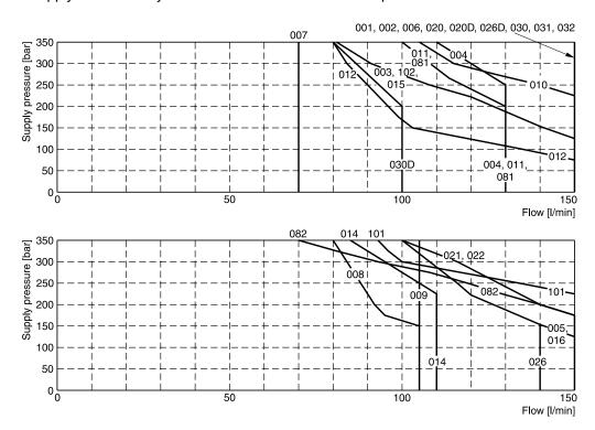
Measured with HLP46 at 50 °C, 90 %  $U_{\tiny nom}$  and warm solenoids.
