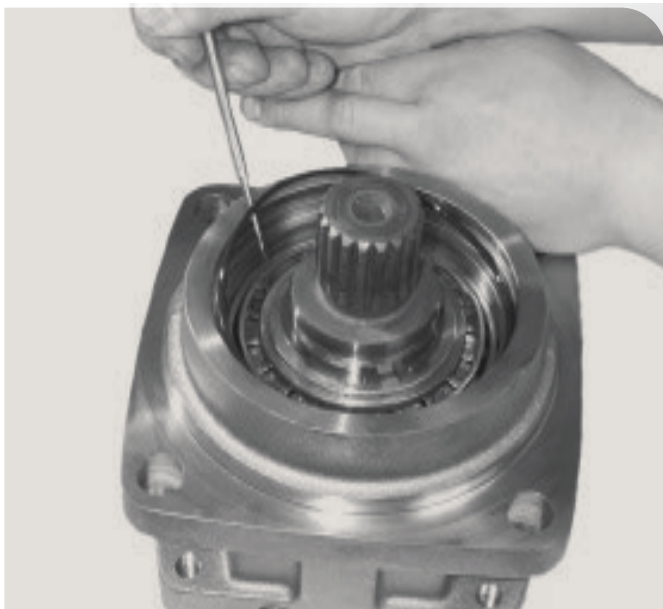
15. Remove the O-ring.
