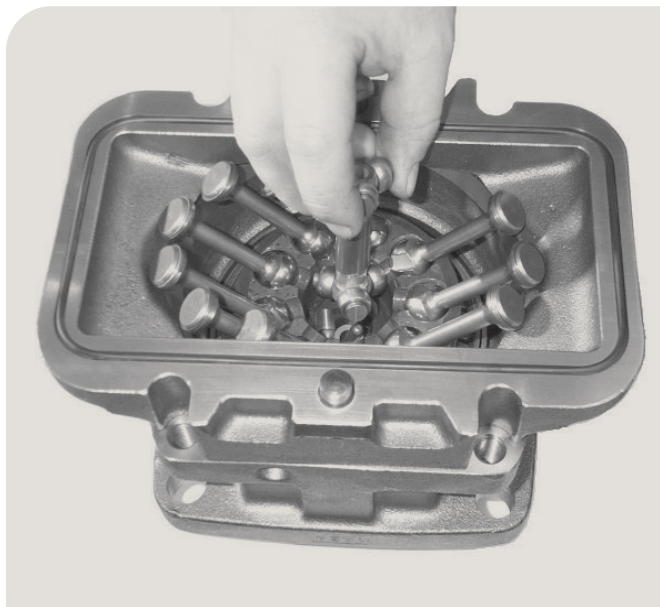
14. Assemble the joint shaft. Put some grease on the joint shaft so the rollers don't fall off. Assemble the rollers with the chamfer inwards.
