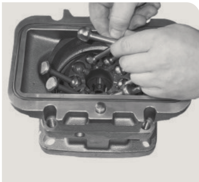
11. Remove the pistons and the O-ring fitted on the intermediate housing.
