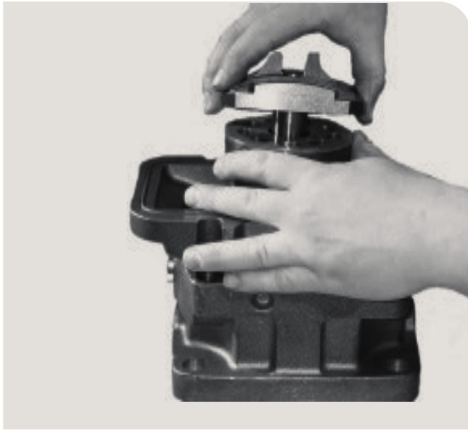
5. Lift the valve segment.
