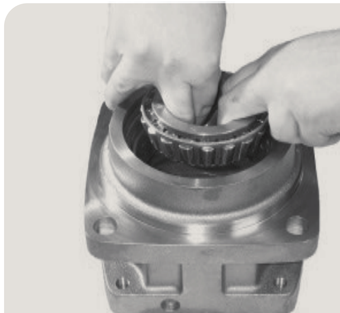
18. Lift the bearing.
