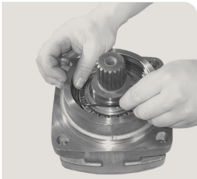
5. Assemble the O-ring.
